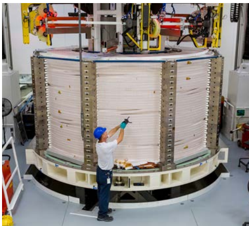
Turn insulation of module nearing completion
