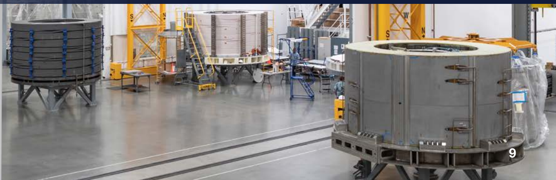
Four ITER CS production modules in various stages of fabrication, from left, prepping the module for vacuum pressure impregnation, following heat treatment, post-turn insulation and fabrication complete, prepared for testing.
