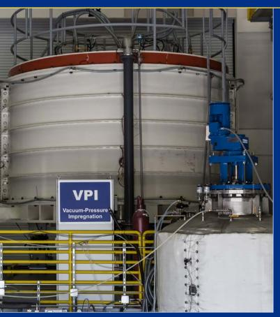
Module mold alongside resin tanks and mixing pump system for injecting 3,500 liters of resin to encapsulate the module
