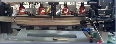
Welding stainless steel cover over the splice joint
