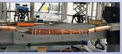
Splicing the conductor cable together similar to splicing a rope
