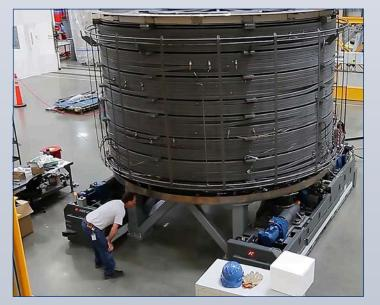
Technician inspecting module after heat treatment
