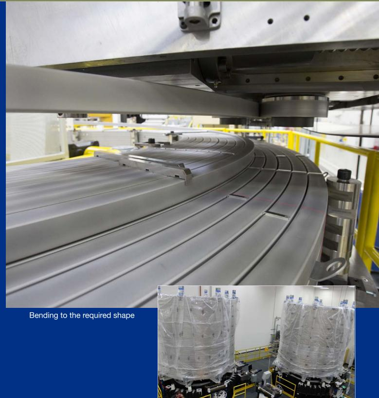
Each Central Solenoid module will be fabricated from approximately 6,000 meters of niobium-tin (Nb<sub>3</sub>Sn) conductor. The production module segment here is wound from 900 meters of conductor into 14-turn pancakes with six layers.
