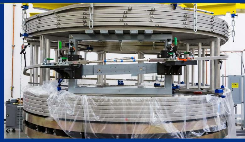
Two hex submodules prepared prior to joining
