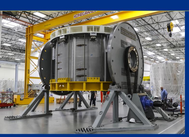
Modules require rotation to exchange bases under coil and allow access for piping installation
