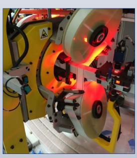
Automated heads wrapping fiberglass tape around the conductor
