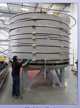
Module with six completed splice joints
