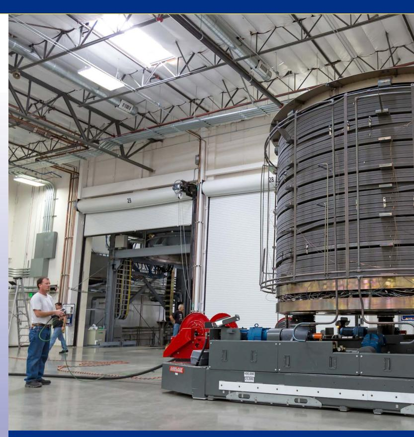
Moving 250,000 lb. (110-tonne) module in facility requires air transporter
