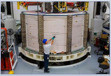
Turn insulation of module nearing completion
