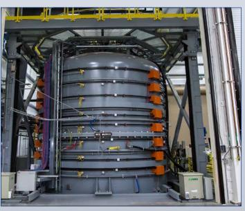
Furnace closed for module heat treatment
