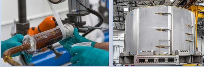
Thirty-nine helium pipes welded and insulated to provide the supply and return for supercritical helium at 4.7 K
