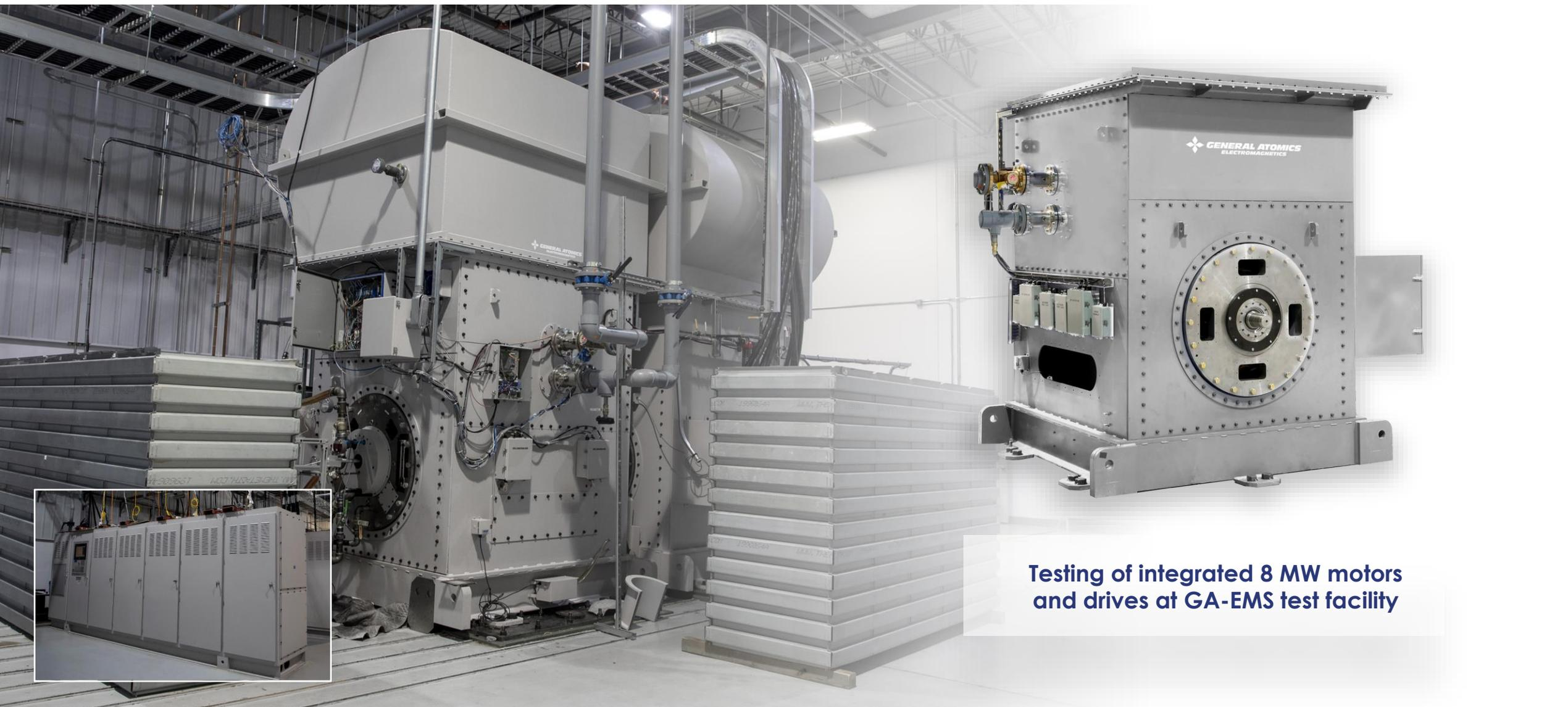
Testing of integrated 8 MW motors and drives at GA-EMS test facility
