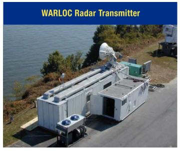
This proof-of-concept long-range radar transmitter used for imaging aircraft produced a 10 kW amplified signal with nearly 1 GHz bandwidth at 94 GHz. (Naval Research Laboratory)
