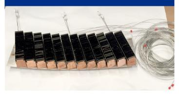
The helicon project is a novel plasma heating system based on a high-power travelling-wave antenna operated in vacuum. The system is designed to deliver over 1 MW at 460 MHz. (Department of Energy)
