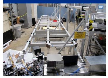
This key microwave-based diagnostic provides real-time data for ITER operations. The system uses a 30-165 GHz frequency-chirped waveform to probe the plasma. (ITER Organization)
