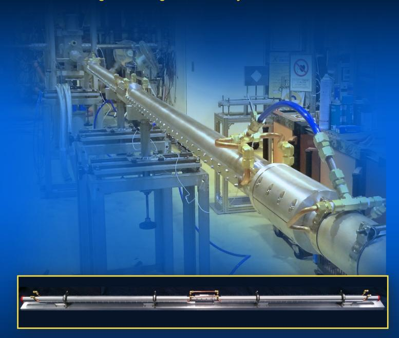
Designed for 1.5 MW, continuous wave operation
