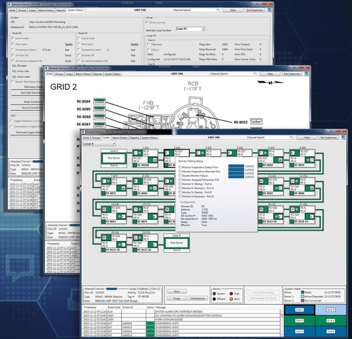
General Atomics Electromagnetic Systems (GA-EMS) RM-11U supervisory computer system provides robust communications capabilities to collect radiation monitor information and display the information at remote consoles in the control room and other locations within a nuclear power plant.
