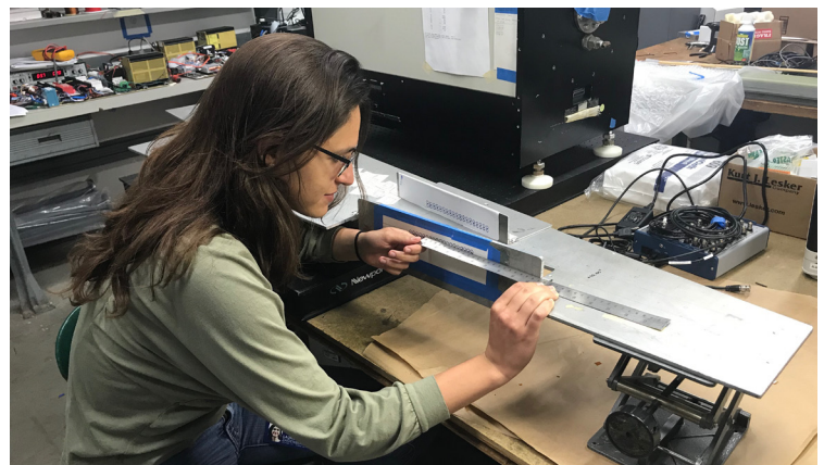
SULI student checks the spatial calibration of a charge exchange recombination spectroscopy system, as part of research into 3-D effects on plasma equilibrium
