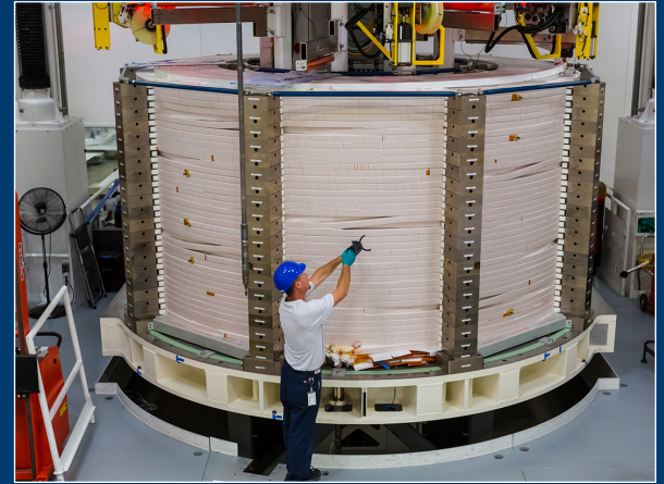
ITER CS module during fabrication
