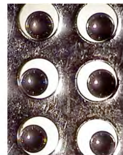
Tungsten-Coated Glass Shells
