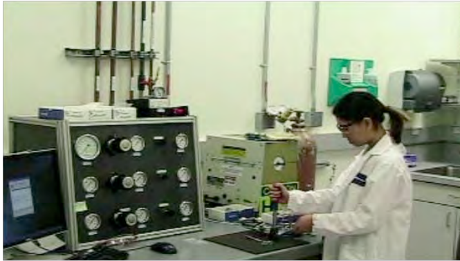
Production gas fill station.
