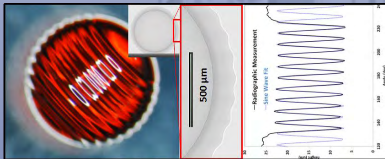
Optical image of ~2 mm OD test capsule with 7.8 μm amplitude ripple
