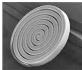
Free-standing spiral machined from tantalum oxide aerogel using 248 nm excimer laser. Diameter of spiral samples is 2 mm.
