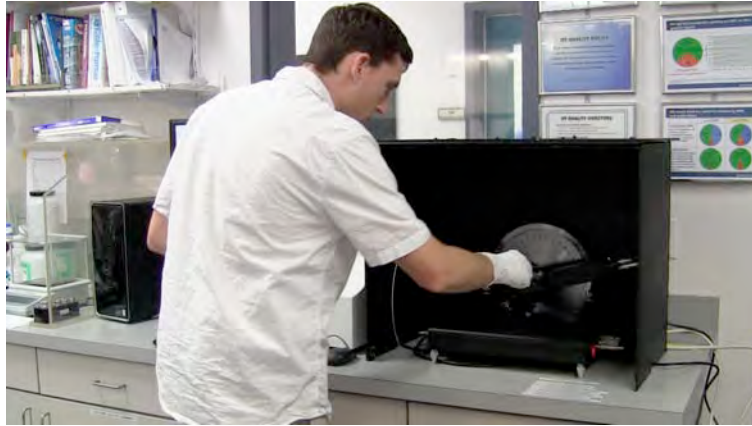
Ellipsometer used to measure pinhole free thin films
