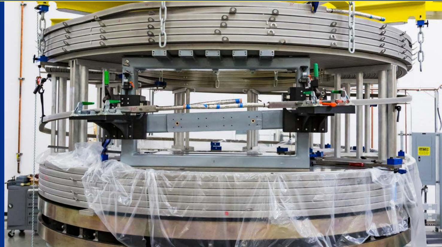
Two hex submodules prepared prior to joining
