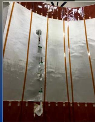
Helium inlet pipe with ground insulation
