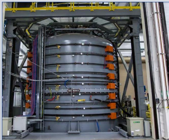
Furnace closed for module heat treatment
