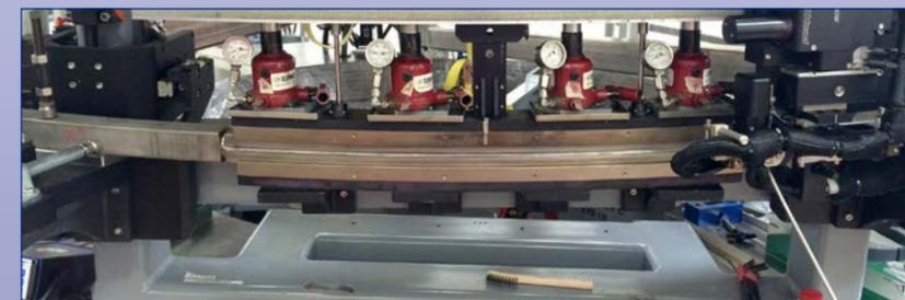
Welding stainless steel cover over the splice joint
