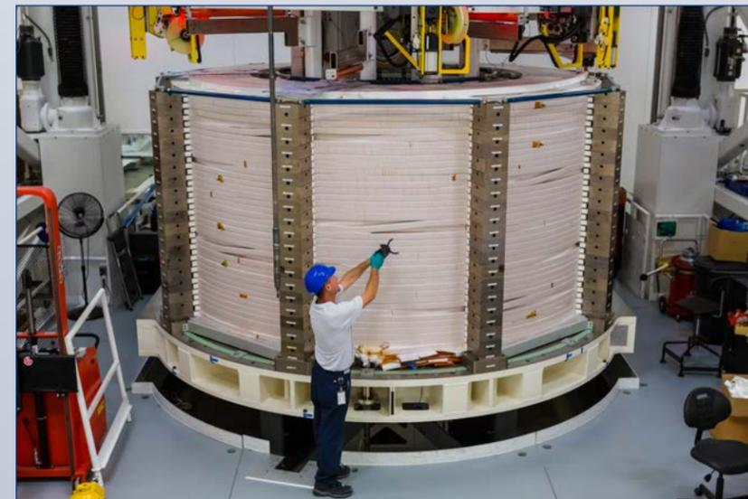
Turn insulation of module nearing completion
