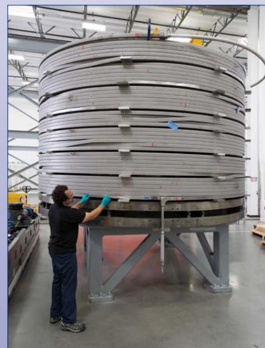
Module with six completed splice joints
