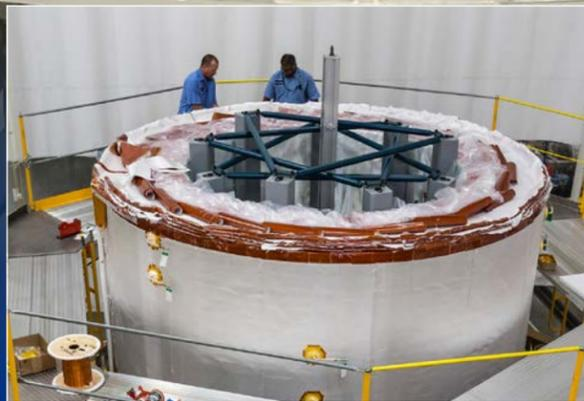
Module during ground insulation application
