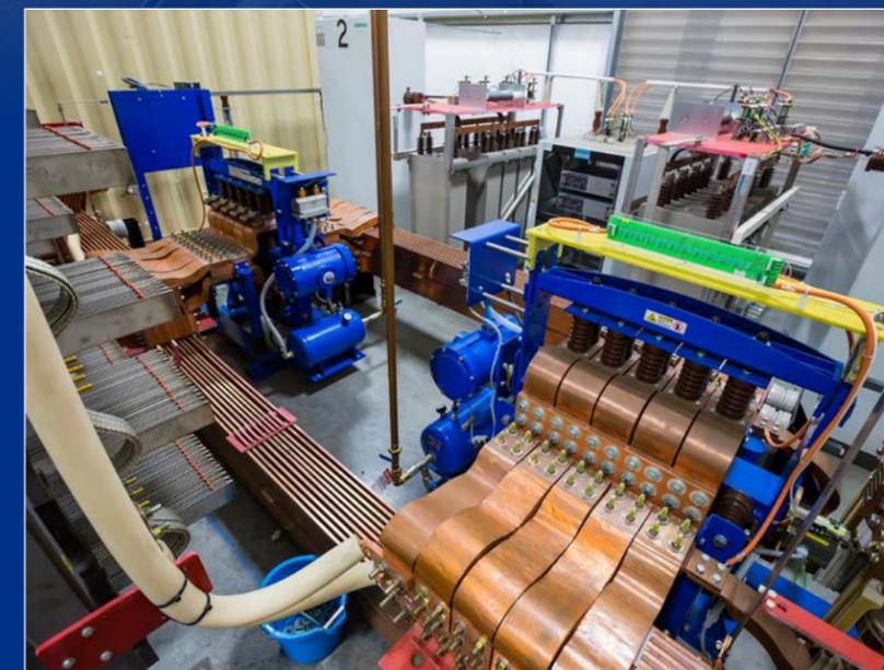
50kA magnet charging power supply with 1GJ fast discharge system including 7kV DC switch and dump resistor for full-current testing of CS modules
