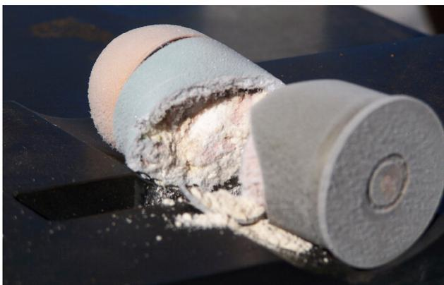
40mm HEPD grenade post cryofracture processing
