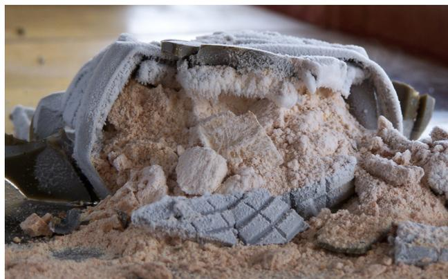
BLU 61A/B (CBU 51B/B) post cryofracture processing
