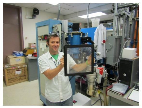
Zachery Seeley holds up a GLO Transparent Ceramic Scintillator, an instrument that dramatically increases high-energy radiography throughput by providing seven times faster imaging than glass scintillators and decreases the X-ray dose required to obtain detailed imagery.
