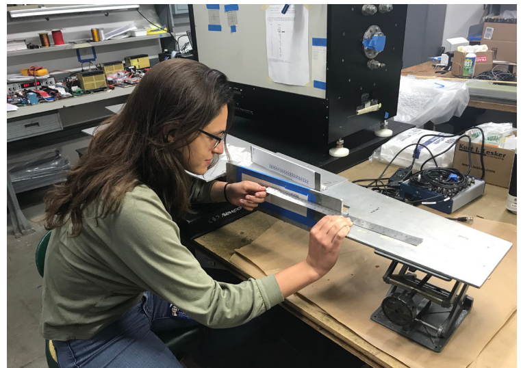
SULI student checks the spatial calibration of a charge exchange recombination spectroscopy system, as part of research into 3-D effects on plasma equilibrium
