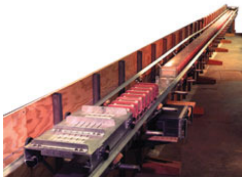
The 20-meter test track at Lawrence Livermore Laboratory used drive coils in its first 4.5 meters for propelling a 20-kg cart to 20 m/s. That was about six times the speed needed to levitate the vehicle.
