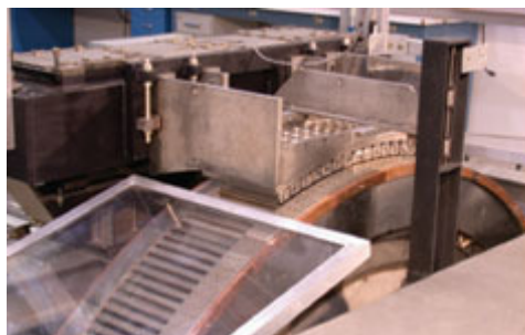
A second-generation test at General Atomics' Dynamic Test Facility holds the cart stationary while the track rolls by below it.
