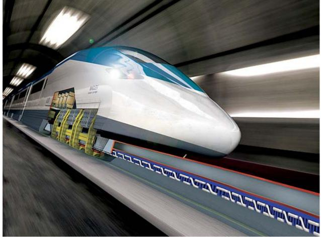
Unlike conventional diesel- and electric-powered trains, the motor for maglev trains is essentially embedded in the track. The track creates a traveling magnetic field beneath the train, which lifts the cars and propels them at 300-plus mph. The train's on-board systems are powered by induction from the track. And only the section of track under the train is energized. (Diagram by Hello-Napalm)
