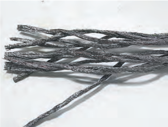
Conductor cable will be coiled at General Atomics in Poway to make a huge electromagnet for the ITER Tokamak in southern France. HAYNE PALMOUR IV • U-T PHOTOS
