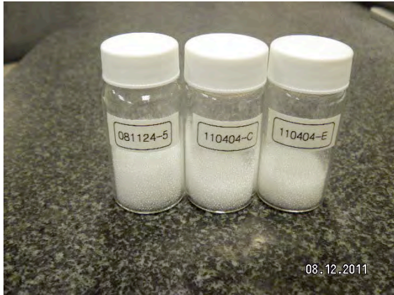
Vials of mass-produced PAMS shells.
