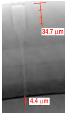
Example of high aspect ratio laser-drilled counter bore hole in beryllium shell.
