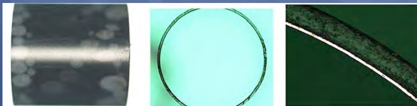
(a) Side view of FeK Shell Target Cylinder. Cylinder is approximately 4 mm in length and diameter. SS-304 (70 atom% Fe) coating was deposited inside 50 \mu\text{m} wall thickness epoxy. (b) Cross-section of cylinder with Fe coating. (c) High magnification of wall cross-section showing thin Fe inner layer.
