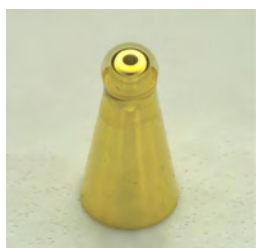
Shock timing cone and shell target.
