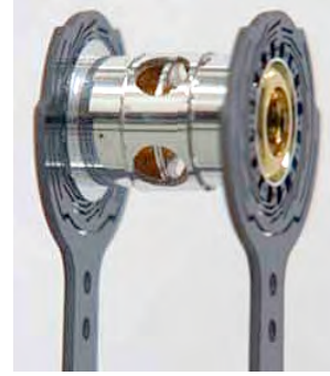
NIF ignition target which includes TMP subassembly.
