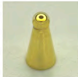
Shock timing cone and shell target
