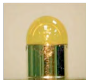
Assembled cryo target with double hemi shell.
