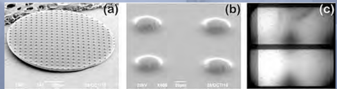
(a) CH flat foil target with square array of bumps. (b) Bumps are nominally 12 \mu\text{m} tall, 25 \mu\text{m} FWHM, and spaced 125 \mu\text{m} apart on a 60 \mu\text{m} thick CH disk. (c) Experimental radiograph from OMEGA shot.
