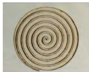
Free-standing spiral machined from tantalum oxide aerogel using 248 nm excimer laser. Diameter of spiral samples is 2 mm.
