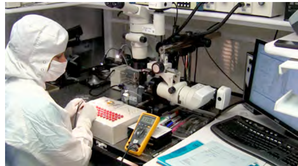
Electrical testing of TMP subassembly.
