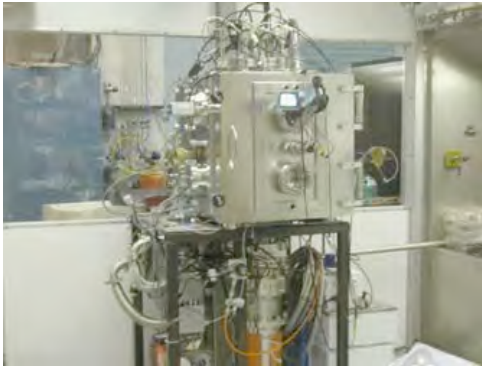
GA coater used for beryllium shell fabrication.
