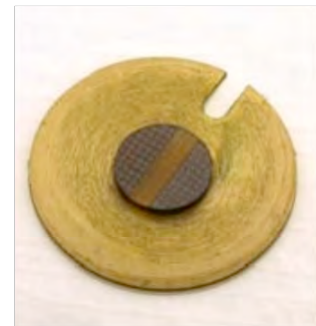
Micromachined BlastWave target.
