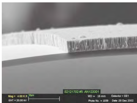
SEM of tungsten coating cross section.
