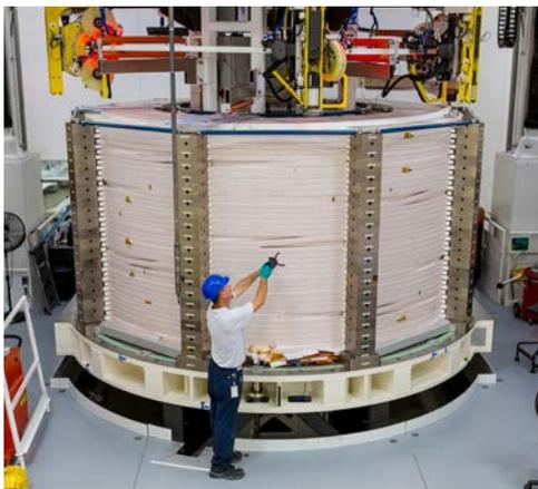
Turn insulation of module nearing completion
