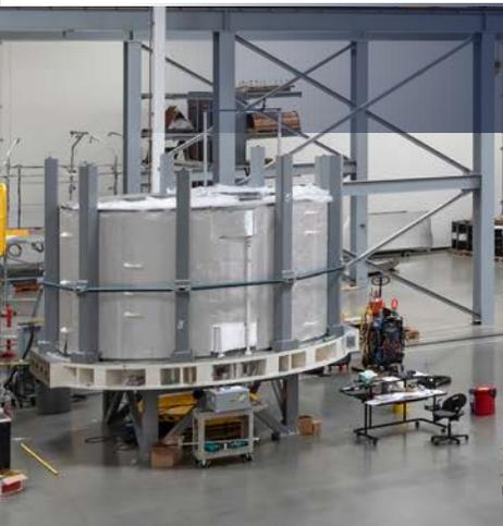
Four ITER CS production modules in various stages of fabrication, from left, prepping the module for vacuum pressure impregnation, following heat treatment, post-turn insulation and fabrication complete, prepared for testing.
