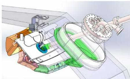
Top-Launch Electron-Cyclotron Current Drive
