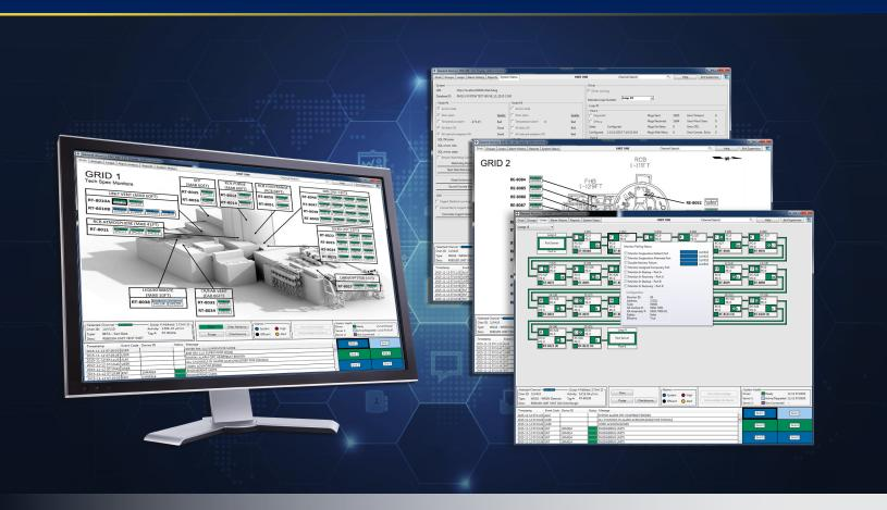
General Atomics Electromagnetic Systems (GA-EMS) RM-11U supervisory computer system provides robust communications capabilities to collect radiation monitor information and display the information at remote consoles in the control room and other locations within a nuclear power plant.
