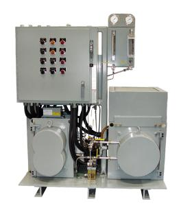
The Sample Detection Skid is located down-stream from the Sample Conditioning Skid. It monitors radioactive gas concentrations over a 12-decade range using three radiation detectors. Each of the two flow paths has separate pumps, valves flowmeters, relays, and control switches. The flow through the monitor is automatically controlled by the RM-2000 Digital Radiation Processor to maintain isokinetic sample flow rates from the Isokinetic Sample Probe Assembly.
