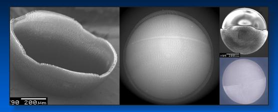
Thin-wall foam hemi mounted on direct-drive capsule
