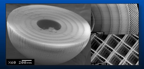
Gradient density foams in spherical geometries
