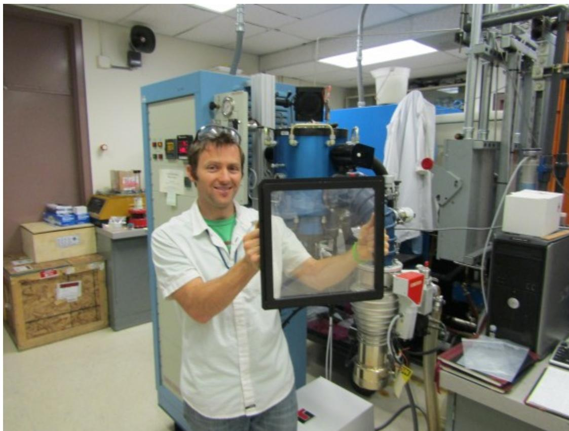
Zachary Seeley holds up a GLO Transparent Ceramic Scintillator, an instrument that dramatically increases high-energy radiography throughput by providing seven times faster imaging than glass scintillators and decreases the X-ray dose required to obtain detailed imagery.
