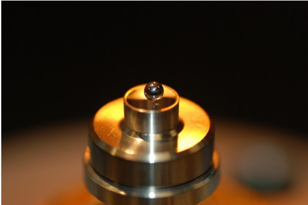
A stainless steel ball is supported by a thin sheet of plastic about 200 atoms thick. The plastic sheet was produced using a technology known as Polyelectrolyte Enabled Liff (PEEL), which was developed by LLNL researchers and General Atomics.
