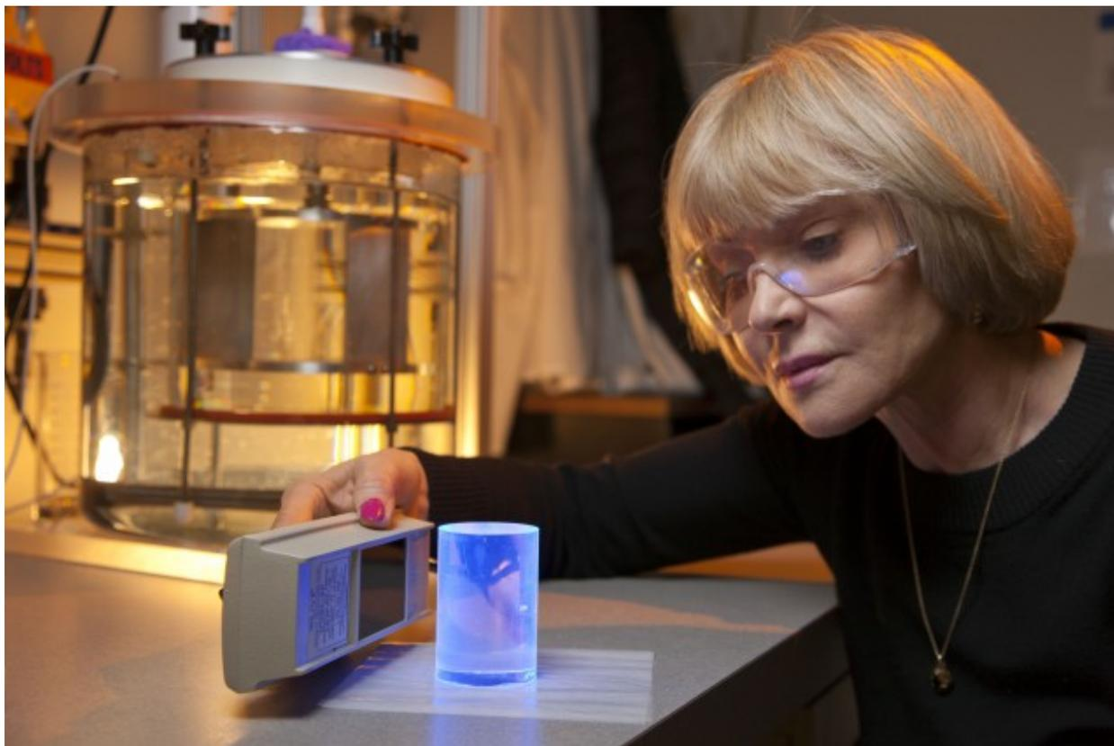
Natalia Zaitseva, an LLNL materials scientist, leads a team of Livermore researchers that has developed the first plastic material capable of efficiently distinguishing neutrons from gamma rays, something not thought possible for the past five decades.
