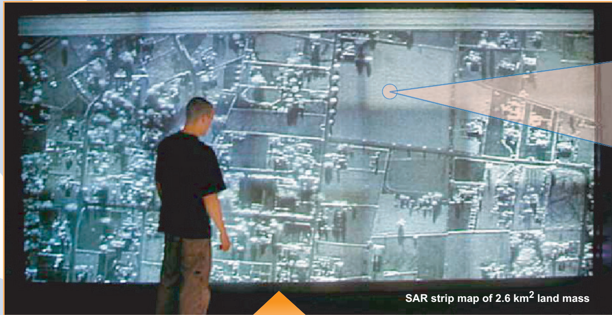
Tiled Display Powered by Parallel Clustered Architecture
