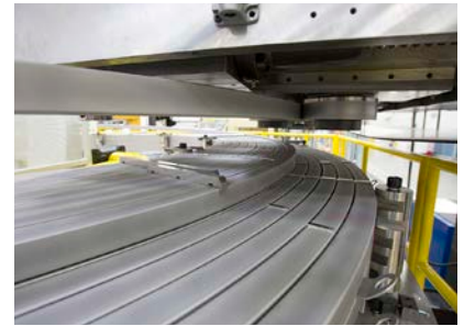
Superconductor is wound to high tolerance
