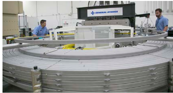
Superconductor is wound to high tolerance
