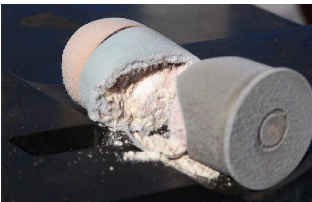
40mm HEPD grenade post cryofracture processing
