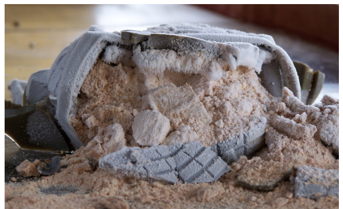
BLU 61A/B (CBU 51B/B) post cryofracture processing
