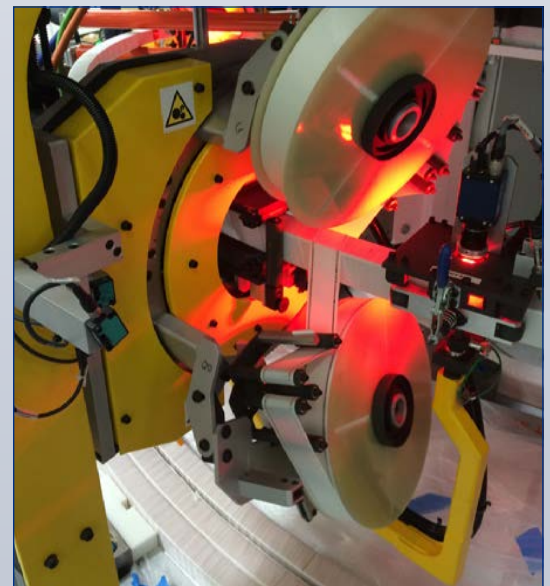
Automated heads wrapping fiberglass tape around the conductor
