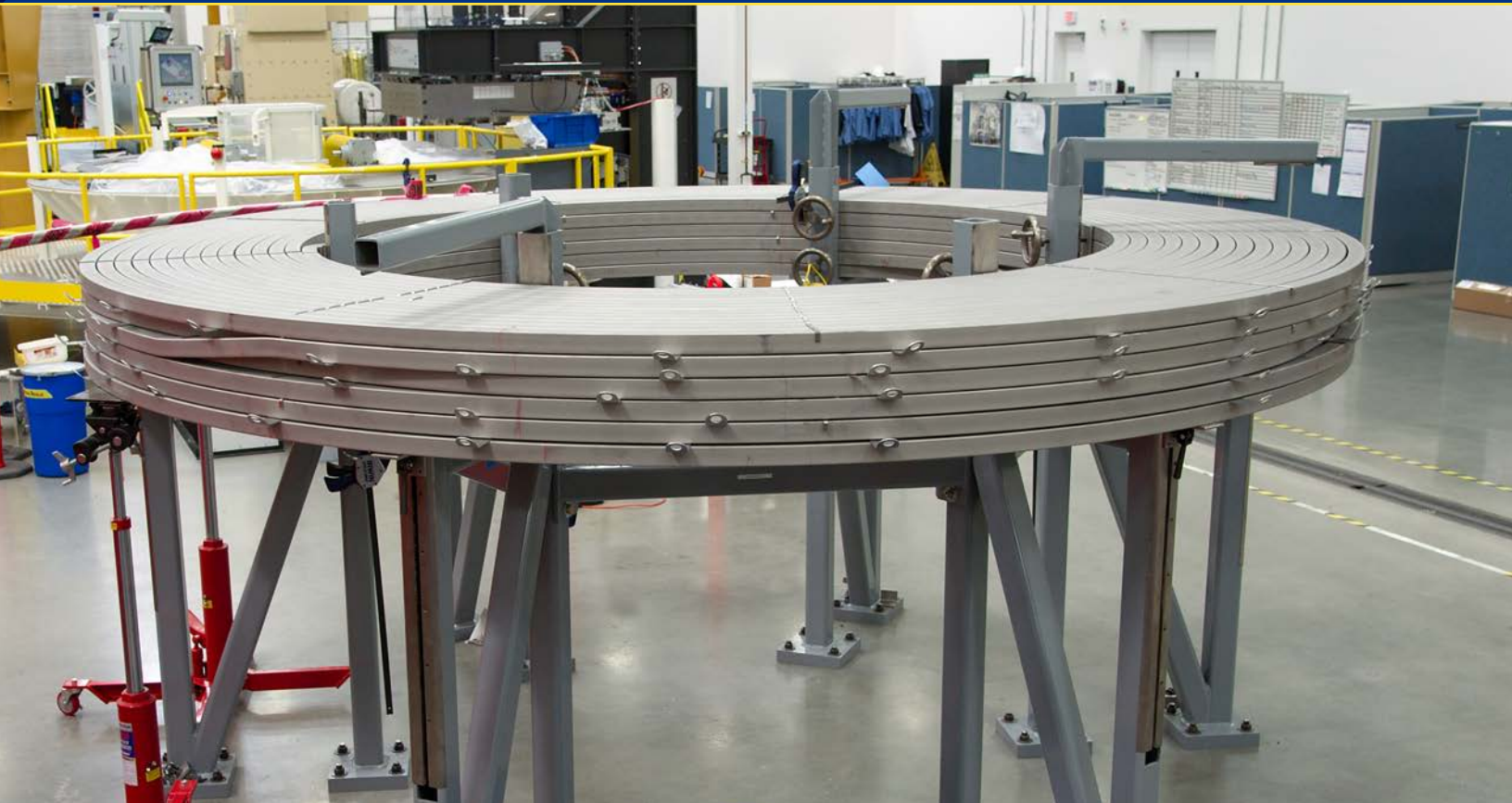
Wound six-layer submodules ready for terminal preparation
