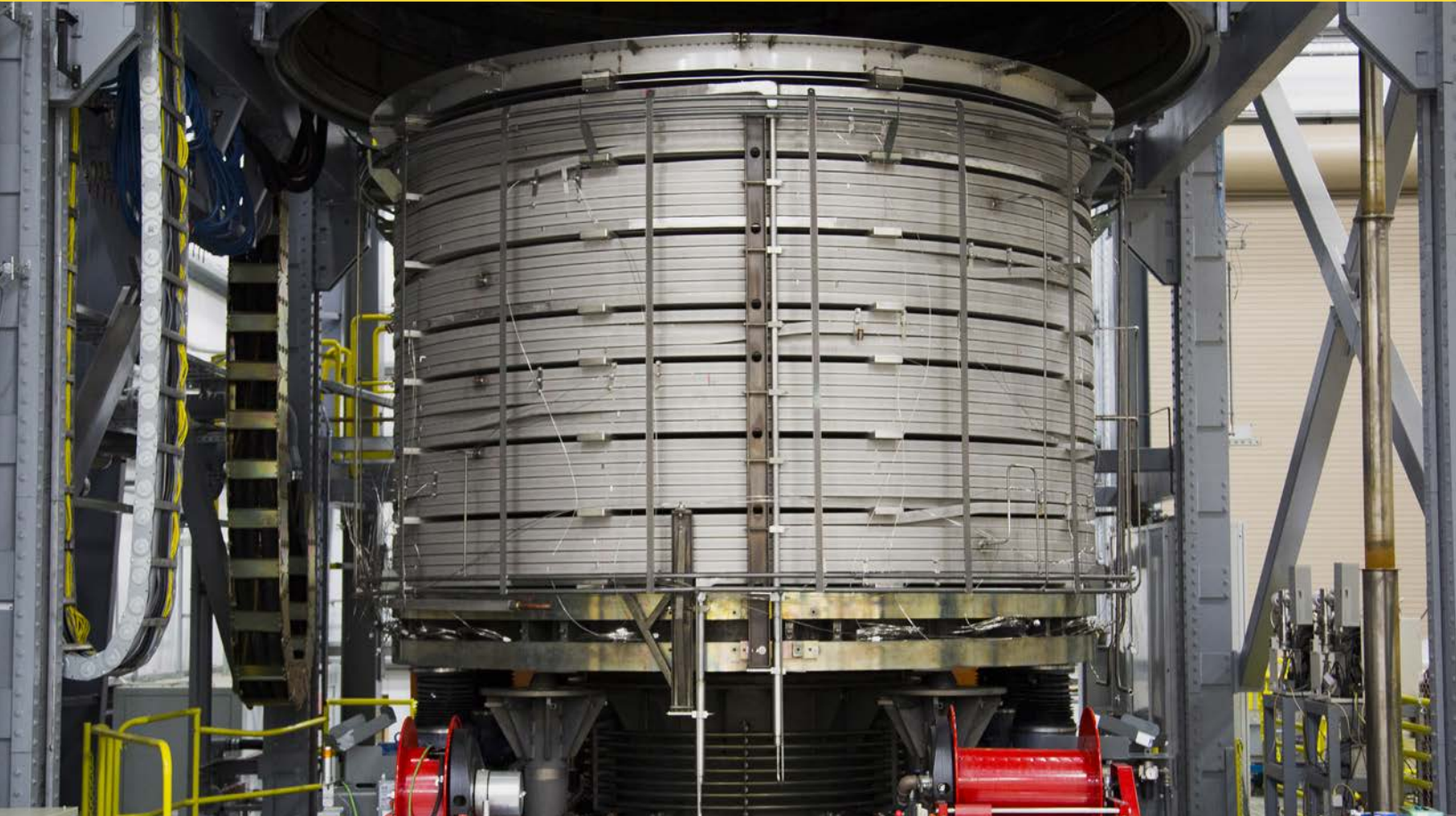
Placing module in furnace for heat treatment at 650°C (1200°F)
