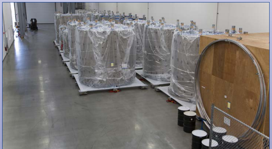
Conductor spools stored prior to winding
