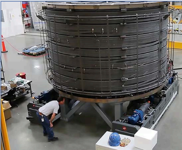
Technician inspecting module after heat treatment
