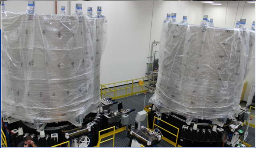
Two spools loaded for winding
