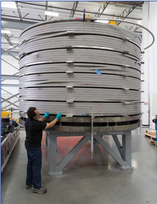
Module with six completed splice joints
