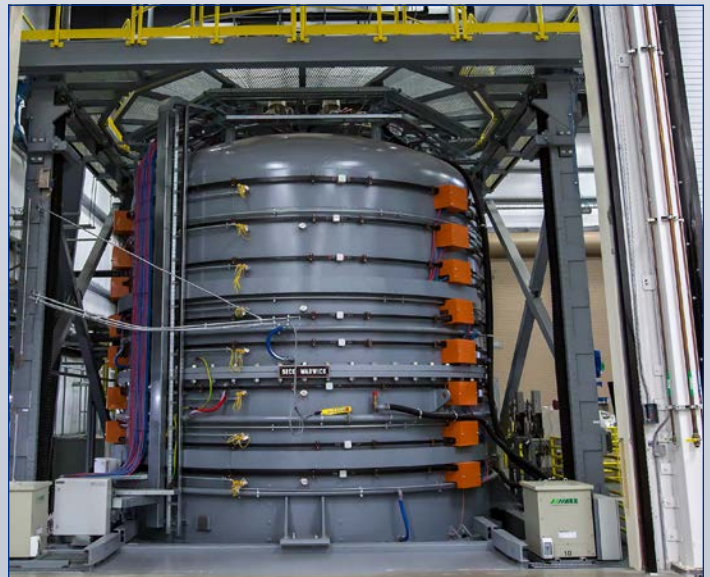
Furnace closed for module heat treatment
