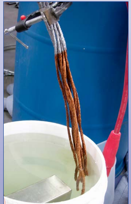
Conductor strands after chrome stripping
