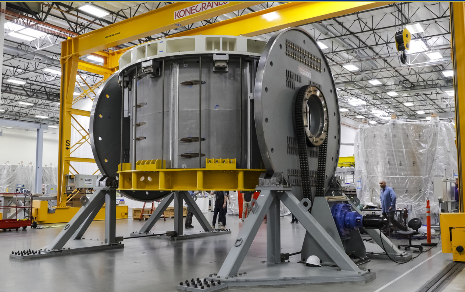
Modules require rotation to exchange bases under coil and allow access for piping installation
