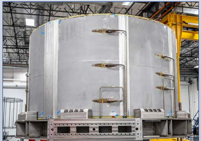
Module after piping installed
