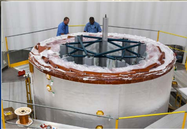
Module during ground insulation application
