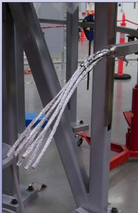
Conductor strands prior to chrome stripping
