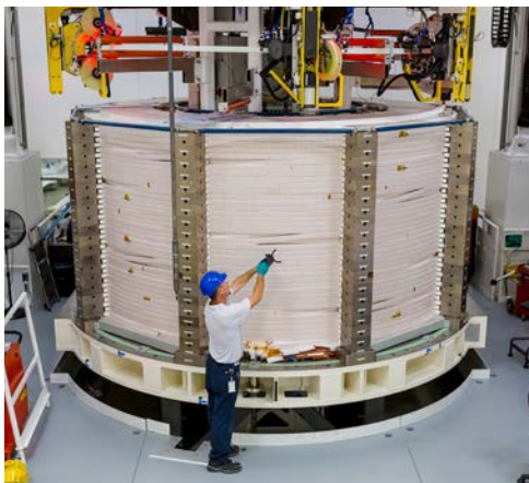
Turn insulation of module nearing completion
